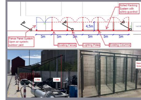
As part of renovation works at CS3-AMC, an oil storage and waste accumulation area have been installed to improve waste management process at site.
